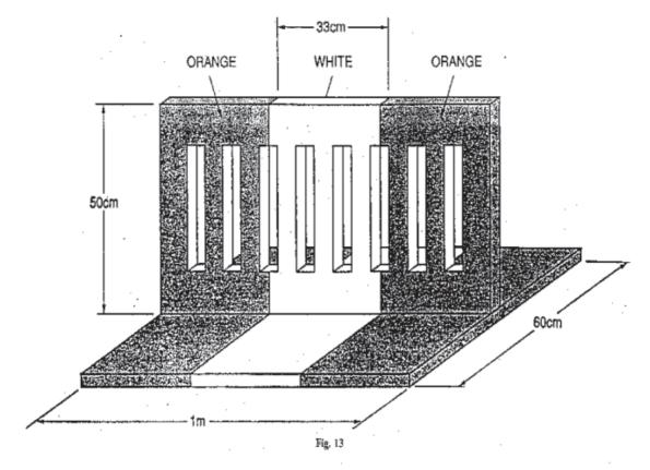
spaced no more than 15 metres apart, signify the boundary of that part of a paved runway, taxiway or apron which is unfit for the movement of aircraft.
