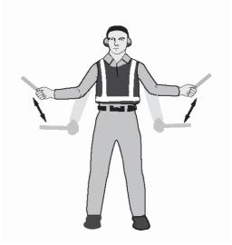
12. With arms down and wands toward ground, wave either right or left wand up and down indicating engine(s) on left or right side respectively should be slowed down. Slow down engine(s) on indicated side
