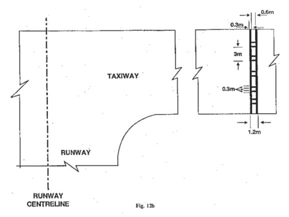
signifies a holding position other than that closest to the runway beyond which no part of a flying machine or vehicle shall project in the direction of the runway without permission from the air traffic control unit at the aerodrome during the notified hours of watch of that unit.
