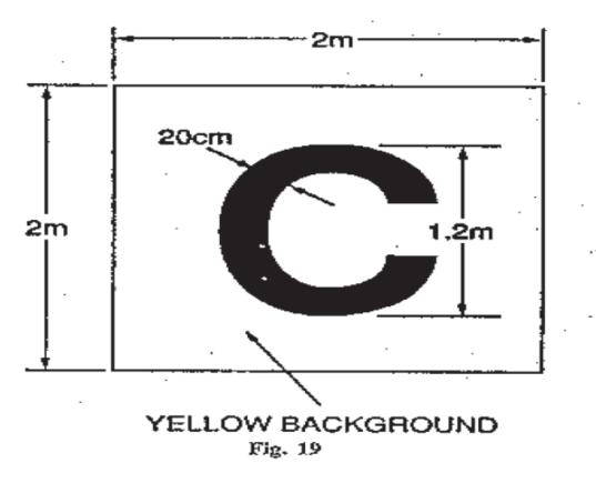
indicates the position at which a pilot can report to the air traffic control unit or to the person in charge of the aerodrome.
