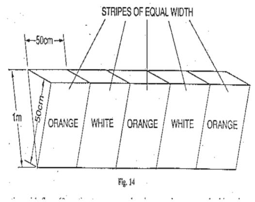
indicate the boundary of an area unfit for the movement of aircraft.
