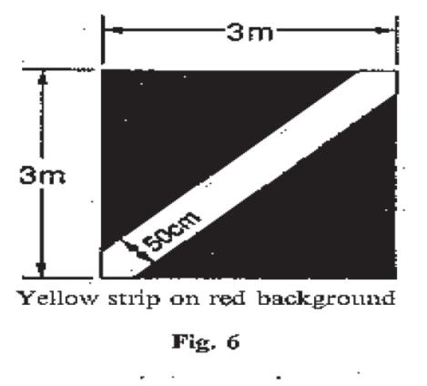
signifies that the state of the manoeuvring area is poor and pilots must exercise special care when landing.
