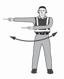
19(b) Extend arm horizontally at a 90degree angle to left side of body. Move other arm in same direction in a sweeping motion. Move horizontally right (from pilot's point of view)
