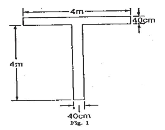
signifies that aeroplanes and gliders taking off or landing shall do so in a direction parallel with the shaft of the T and towards the cross arm, unless otherwise authorised by the appropriate air traffic control unit.
