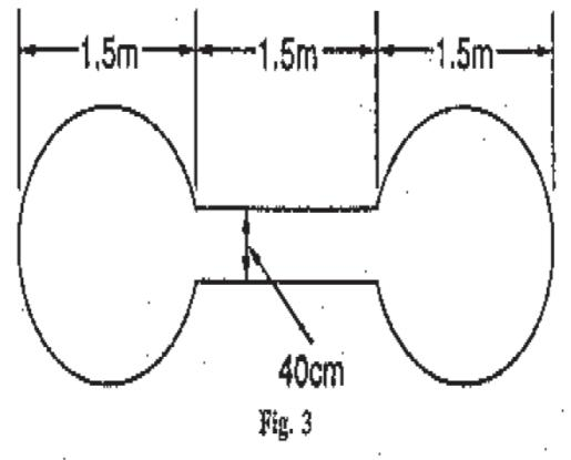
signifies that movements of aeroplanes and gliders on the ground shall be confined to paved, metalled or similar hard surfaces.
