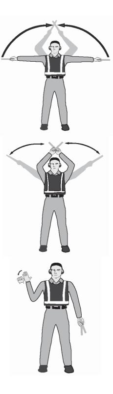
7(b) Raise hand just above shoulder height with hand closed in a fist. Ensuring eye contact with flight crew, open palm. Do not move until receipt of "thumbs up" acknowledgement from crew. Release brakes
