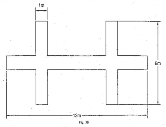
indicates an area which shall be used only for the taking off and landing of gliders.
