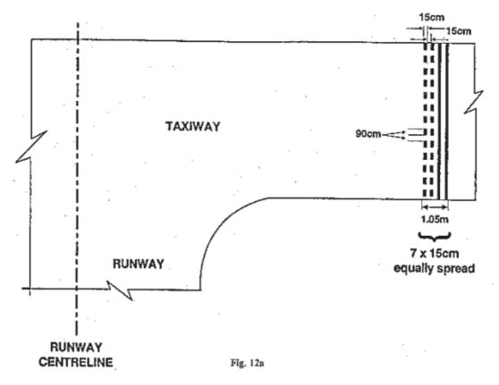
in this paragraph, signify the designated visual holding position associated with a runway beyond which no part of a flying machine or vehicle shall project in the direction of the runway without permission from the air traffic control unit at the aerodrome during the notified hours of watch of that unit.
