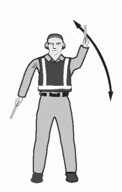
15. Raise right arm to head level with wand pointing up or display hand with "thumbs up"; left arm remains at side by knee. Affirmative/all clear— This signal is also used as a technical/servicing communication signal.
