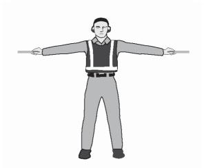
17. Fully extend arms and wands at a 90-degree angle to sides and, with palms turned up, move hands upwards. Speed of movement indicates rate of ascent.
