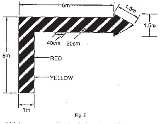
the shaft of which is one metre wide and which is placed along the whole or a total of 11 metres of two adjacent sides of the signals area, and pointing in a clockwise direction, signifies that a right-hand circuit is in force.
