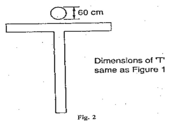
signifies that the direction of landing and take off do not necessarily coincide.
