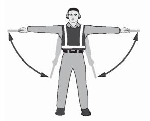
19(a) Extend arm horizontally at a 90degree angle to right side of body. Move other arm in same direction in a sweeping motion. Move horizontally left (from pilot's point of view)
