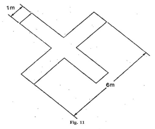
displayed on a runway or taxiway, with each arm of each cross at an angle of 45° to the centre line of the runway, at intervals of not more than 300 metres signify that the section of the runway or taxiway marked by them is unfit for the movement of aircraft.
