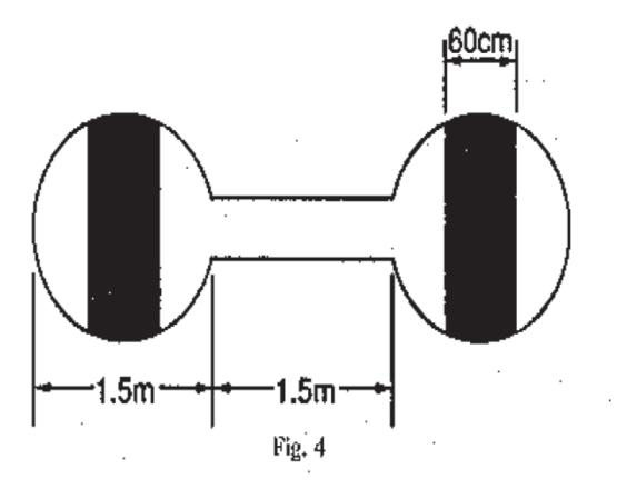
signifies that aeroplanes and gliders taking off or landing shall do so on a runway but that movement on the ground is not confined to paved, metalled or similar hard surfaces.
