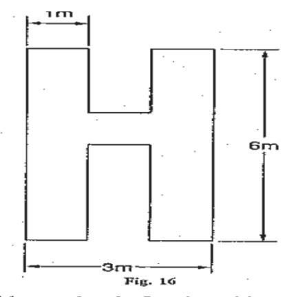
indicates an area which shall be used only for the taking off and landing of helicopters.
